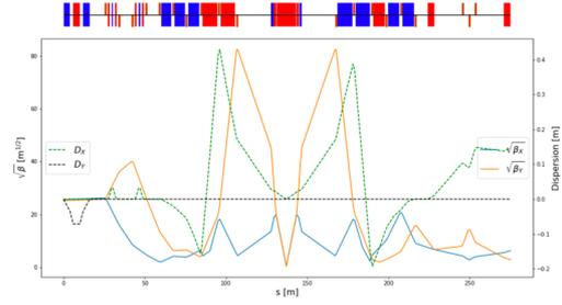
**Figure 6:** Optical functions of the electron beam in the IR.
