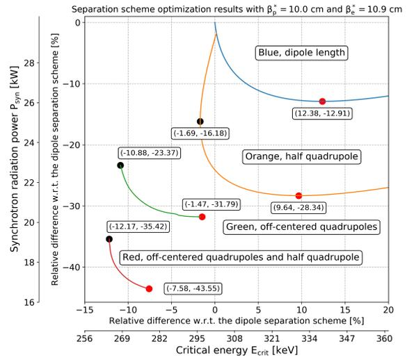
**Figure 7:** Optimising the synchrotron light for lowest critical energy and power, details in the text.
