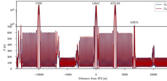
**Figure 4:** LHC proton beam optics, optimised for the LHeC design values of  $\beta=7$  cm at the LHeC IP.
