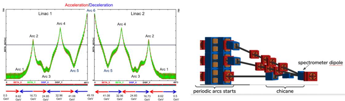
**Figure 3:** Optics functions in the linacs (left): Dispersion suppressor and matching section are connected on both sides to the arc structures via spreader/re-combiner modules (right).
