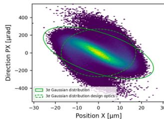
**Figure 8:** Simulation of the beam-beam effect for the electrons plotted in phase space coordinates,  $x, x'$ .
