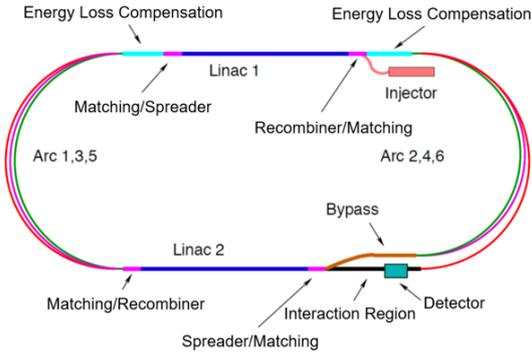
**Figure 1:** Sketch of the ERL geometry, using two sc. linear accelerators, connected by return arcs.
