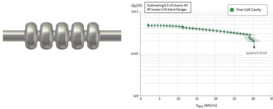
**Figure 2:** Prototype of the superconducting 5 cell cavity and measured quality factor.
