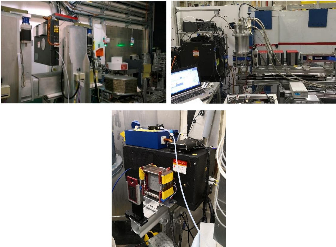
Figure 4. Left, the large in situ ^3\text{He} system installed on MAGREF at SNS as the analyzer; Right, the medium system used as the analyzer on CG-1D at HFIR. Bottom, the compact system set up on HB-3A as the polarizer
