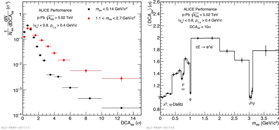
**Figure 5:**  $DCA_{ee}$  spectra in the  $\pi$ -mass region and the IMR normalised to unity (left) and the  $\langle DCA_{ee} \rangle$  as function of  $m_{ee}$  in p–Pb collisions at  $\sqrt{s_{NN}} = 5.02$  TeV.
