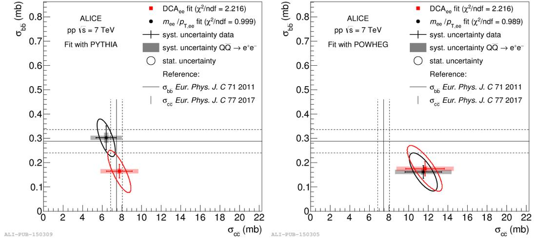
**Figure 3:** Total  $c\bar{c}$  and  $b\bar{b}$  cross sections with systematic and statistical uncertainties, extracted from fits of the measured dielectron yield from heavy-flavour hadron decays to  $(m_{ee}, p_{T,ee})$  and to  $DCA_{ee}$  with PYTHIA (left) and POWHEG (right) in comparison with published cross sections from independent measurements (lines) [1].
