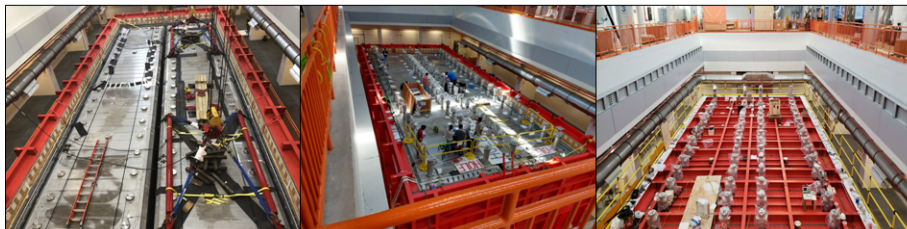
Figure 1: Left: inner view of one ICARUS module with the two TPCs separated by the common central cathode and the new 8" PMT system behind the wire planes, during refurbishing in a CERN clean room. Center: one of the new cold vessels in a CERN workshop. Right: sketch of the layout of the Icarus CRT and picture of bottom CRT panels.
