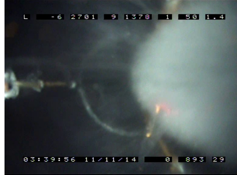
Figure 1. Camera image looking downward into the hole ice. The bubble column is found on the center right.
