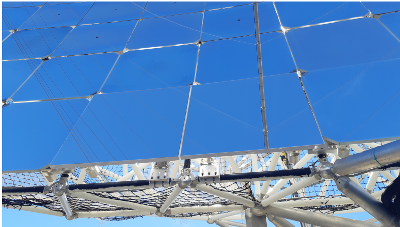
Figure 4: Two mirrors, IDs 227 and 228, were installed in the MAGIC-II telescope in October 2018 to evaluate their performance and long-term behavior under actual on-site condition.
