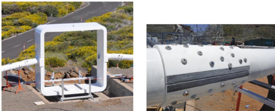
**Figure 2:** The CFRP camera frame during assembly with the CSS (left) and one of the junctions between two sections of the CSS (right).
