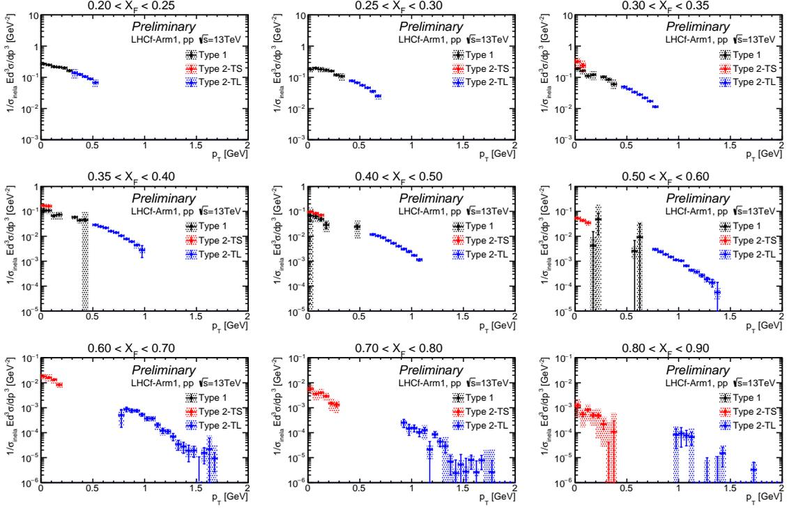
**Figure 5:** The  $\pi^0$  production cross-section as functions of  $p_T$  and  $X_F$  of  $\pi^0$ 's, measured by the LHCf-Arm1 detector at  $pp$ ,  $\sqrt{s} = 13\text{TeV}$ . The error bars and hatched areas indicate statistical and systematic uncertainties, respectively.
