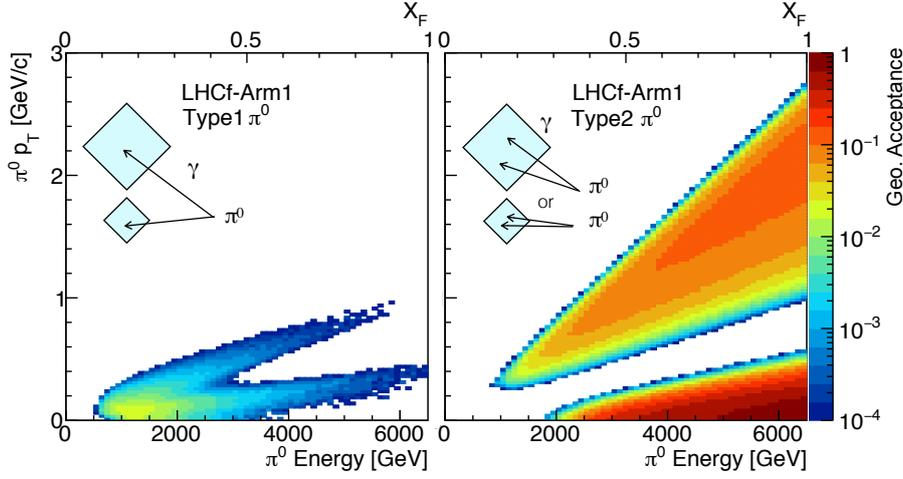
**Figure 3:** Geometrical acceptance of  $\pi^0$  detection by the LHCf-Arm1 detector assuming as the energy threshold of photon detection is 200 GeV. The left and right panels show for Type 1 and Type 2  $\pi^0$  events, respectively.
