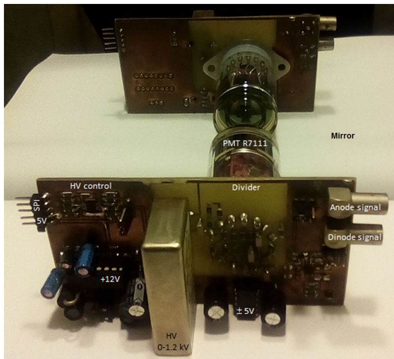
Figure 2: Portable UV detector contains one R7111 photomultiplier tube from the Hamamatsu company.
