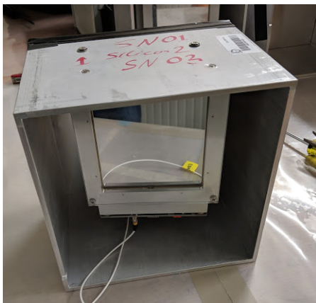
Figure 4: The mounting of two calibration silicon detectors in their lightbox.
