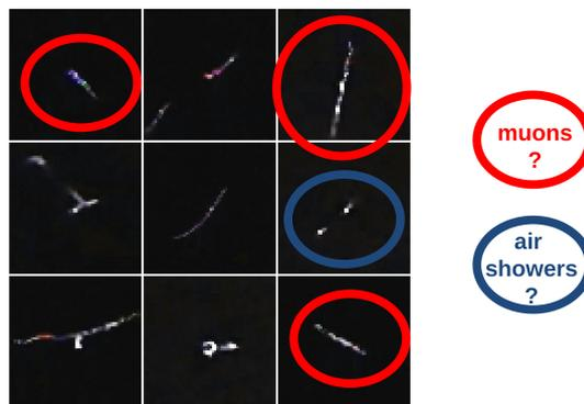
**Figure 3:** The variety of particle tracks candidates as registered by a smartphone using the CREDO Detector app [6].
