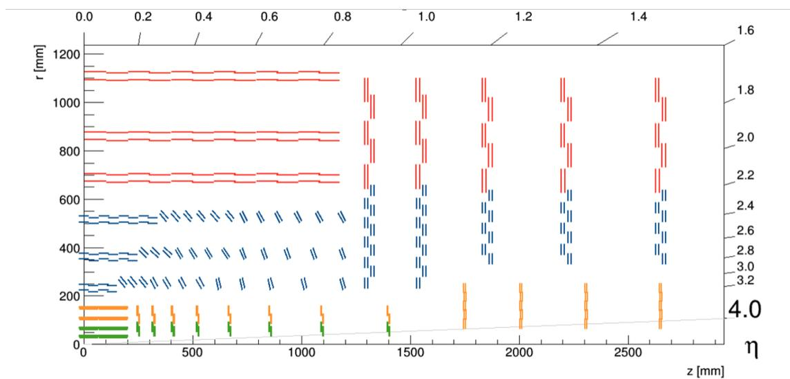
**Figure 1:** Sketch of one quarter of the Phase-2 CMS tracking system in  $r$ - $z$  view. The pixel detector is shown in green/yellow, while single-sided and double-sided strip modules are depicted as red and blue segments, respectively.
