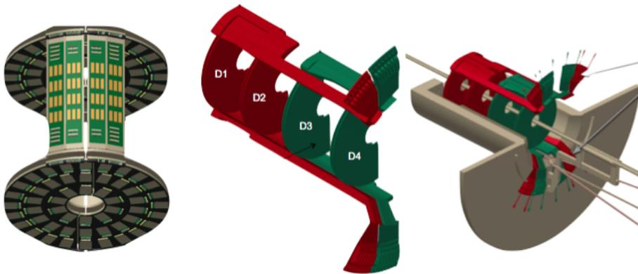
**Figure 3:** Left: Readout electronics arrangement at the top (bottom) of the half quadrant. Center: TEPX quadrant. The two halves are independent because of space constraint during the installation. Right: Rendering of two quadrants after installation in CMS TBPX
