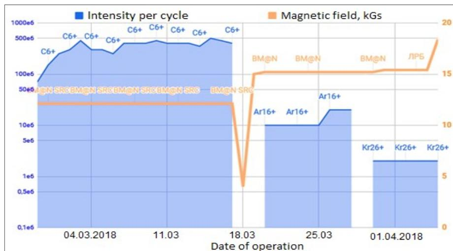
**Figure 5.** Ion species, intensities and the Nuclotron run schedule in spring 2018 run.
