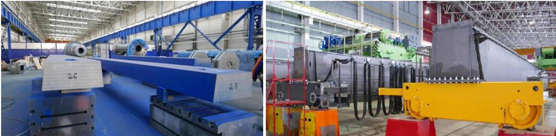
Figure 9. Manufactured 25 from 28 of yoke plates: 0.35x0.74x8.47, m3; 16 tons each are ready (left part). Two 80 ton cranes for the MPD and SPD halls were prepared and tested (right part).
