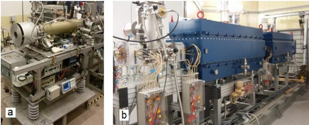
**Figure 6.** Special ion source prepared for heavy ion run at linac LU-20 and Nuclotron for the BM&N setup data taken (a) and the new linear accelerator HILAC for NICA heavy ion injection chain (b).
