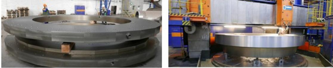
Figure 8. Support rings of 6.63 m diameter, 43.7 tons weight each (left part) and poles 4.5 m diameter, 47 tons each (right part).
