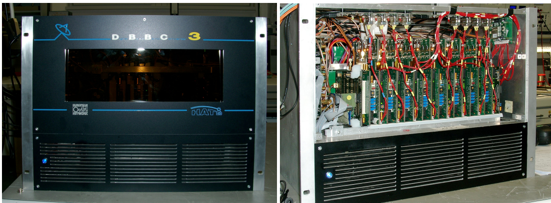
Figure 2: Left: DBBC3 front view. Right: DBBC with 8 IFs, front opened.
