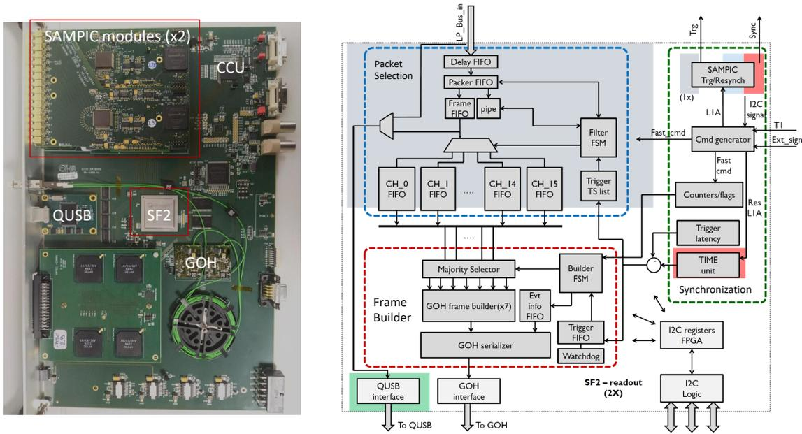
**Figure 1:** On the left a picture of the Digitizer Board fully equipped. A second mezzanine is present at the bottom of the board, hosting the TDC chips used in the PPS project. On the right a scheme of the readout section of the firmware developed for the SF2 FPGA.
