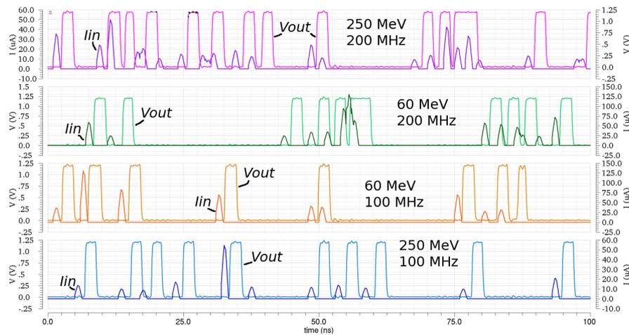
**Figure 4:** CSA channel simulations after layout parasitic extraction.
