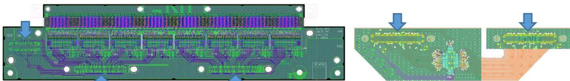
Figure 4: Layout of a hybrid with 8 CBC3/CBC3.1 ASICs (left), and a layout of a CIC mezzanine flex-rigid board (right). Blue arrows point at the footprints of the fine pitch connectors.
