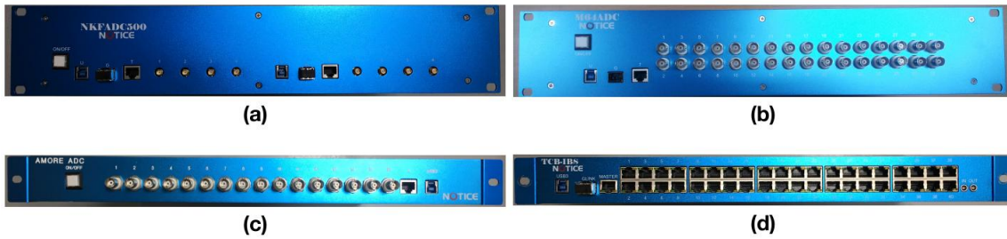
Figure 1: Electronics of CUP DAQ system, (a) FADC500, (b) M64ADC, (c) AMOREADC, (d) TCB.
