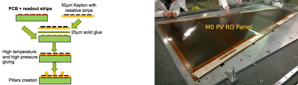
Figure 5: Left: the readout board is made of FR4 PCB with cooper strips coupled with 50 \mu\text{m} Kapton foils with resistive strips by means of 25 \mu\text{m} thin film of solid glue. By high temperature and high pressure the two foils stick together. On top of the resistive strips is glued a Pyralux coverlay from which a regular structure of pillars are made lithographically. Right: readout panel for SM1 module zero.
