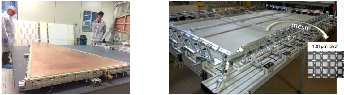
Figure 6: Left: the drift panel with the extruded mesh bars glued ready to be finalized with mesh. Right: stretching of the mesh.
