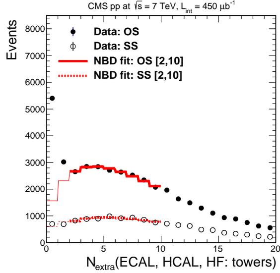
**Figure 2:** Distribution of the multiplicities of ECAL+HCAL+HF towers above noise thresholds,  $N_{\text{extra}}$ , in events with two opposite-sign (solid circles) and same-sign (open circles) tracks [6]. The negative binomial distributions used to reproduce the backgrounds in OS (solid curve) and SS (dashed curve) events are shown in their fitting range (thick lines), as well as their extrapolation below that range (thinner lines).
