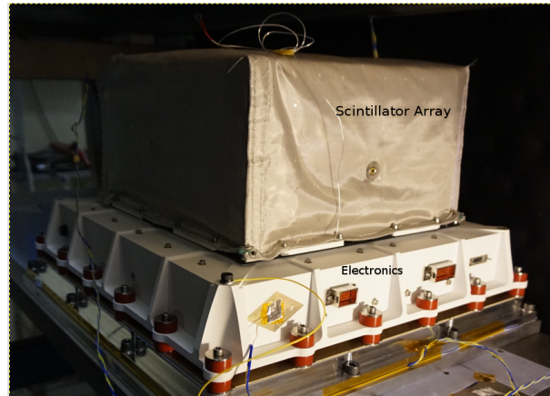
Figure 2: The POLAR flight model during thermal vacuum tests. The electronics is contained in the white painted aluminum structure while the scintillator array is placed in a carbon structure covered with a multi-layer insulator.
