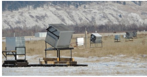
Figure 1: Left: The Layout of the 2017 HiSCORE TAIGA array (satellite picture by google-earth). Right: 3 HiSCORE stations with their electronic boxes.
