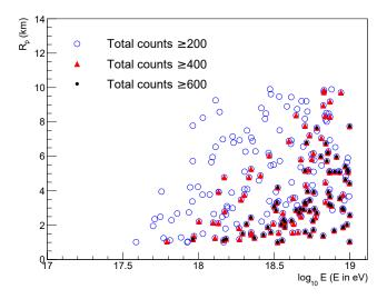
**Figure 3:** Events expected in the EUSO-TA FOV with total counts higher than 200, 400 and 600, respectively 229, 118 and 67 events out of 1000 simulated events. Here, a cosmic ray power spectrum with slope  $E^{-1}$  has been considered, that leads to more events at the high energies than with the actual slope of about  $E^{-3}$ .
