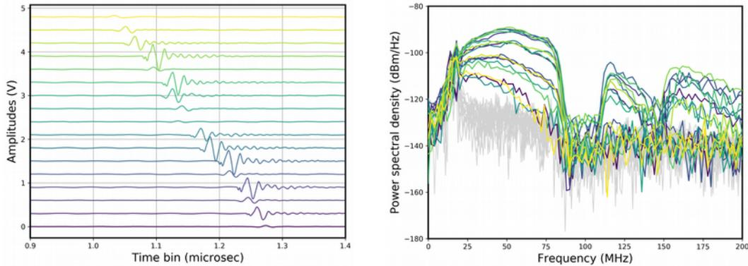
Figure 3: Waveforms (left) observed in the 17 EW antennas of the left-most event of Figure 2. The waveforms are arbitrarily shifted in time and in amplitude for readability. The corresponding PSD (right) are calculated in a time window centered around the transients and compared to noise reference levels (light gray lines).
