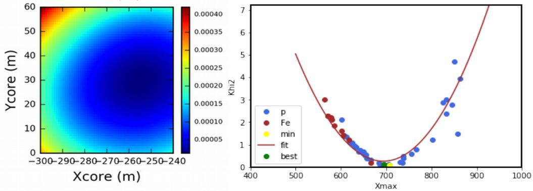
Figure 6: Left:  $\chi^2$  map used to deduce the core location (here around  $x=-250\text{m}$  and  $y=30\text{m}$ ) for a simulation of the same experimental event (on the right of Figure 2). Right: distribution of  $\chi^2_{\min}$  versus  $X_{\max}$  for the entire set of simulations.
