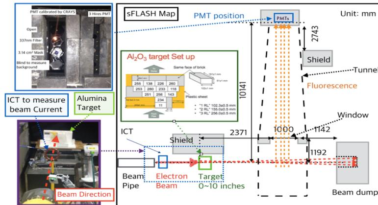
Figure 2. Right) Map of sFLASH configuration, Left top) a picture of PMT setup, sFLASH used 7PMTs. Left bottom) a picture of beam exit, the target is  $\sim 2$  m away from beam window and the ICT measured beam charge between beam window and target.
