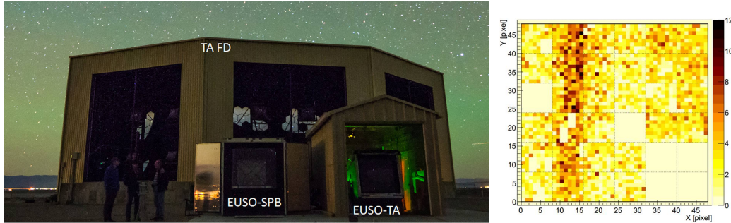
Figure 2: Left: EUSO-TA (front right), main detector of the EUSO-SPB (front left) and TAFD (back) (picture by M. Mustafa). Right: An UHECR event seen by EUSO-TA. An UHECR event of low ( \sim 10^{18} eV) energy traversing at \sim 2.5 km distance from EUSO-TA and therefore visible as a track on a single GTU, in this case going from top-right to bottom-left (distance and energy are estimated by TA). The color scale denotes uncalibrated counts of the detector.
