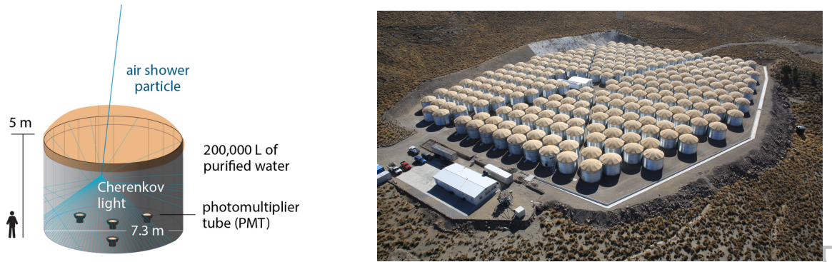
Figure 2: Left: Schematic of the Water Cherenkov Detector with PMT's inside. Right: The HAWC array.
