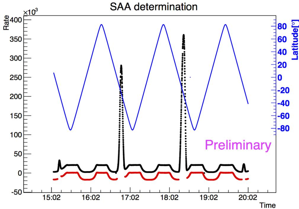
**Figure 1:** The trigger rate during a period when the satellite crosses the SAA 4 times. Black line is the rate before SAA rejection. As the blue line is labeled by latitude, it is clear that top platforms are polar regions and bottoms are equatorial regions. Red line is the rate after SAA rejection. To make a comparison, the red line is shifted down 20000 manually.
