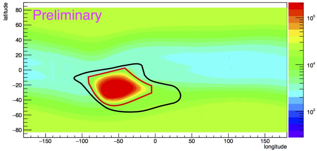
**Figure 2:** The trigger rate variation with geographic latitude and longitude. The red solid line is labeled as the SAA boundary fitted by the data from Jan. 1st to Dec. 31st, 2016. The black solid line is the contour about  $1\text{cm}^{-2}\text{s}^{-1}$  for trapped proton flux above 10 MeV predicted by the AP-9[8].
