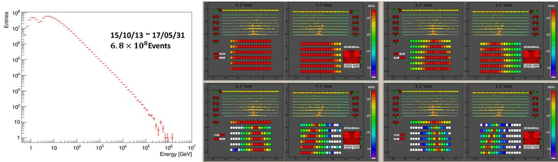
**Figure 5:** Left panel shows TASC energy deposit sum spectrum during October 13, 2015 to May 31, 2017. Right panel represents the highest energy event penetrating whole detectors (about 1PeV). In this panel, top left shows APD high gain view, top right APD low gain, bottom left PD high gain and bottom right PD low gain respectively. It is clearly seen that the four gains cover a whole range of the energy measurements.
