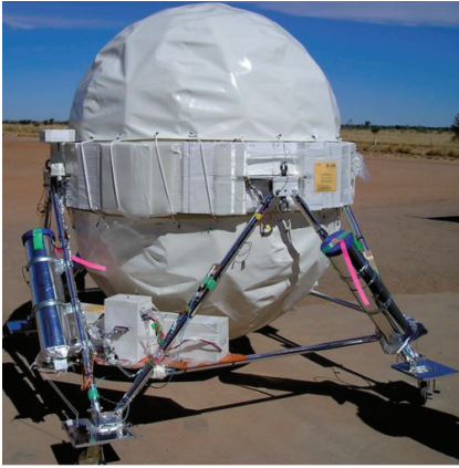
Figure 3: The GRAINE 2015 gondola with thermal shielding. The three star cameras are deployed at the truss structure and each camera views the three different directions of the sky.
