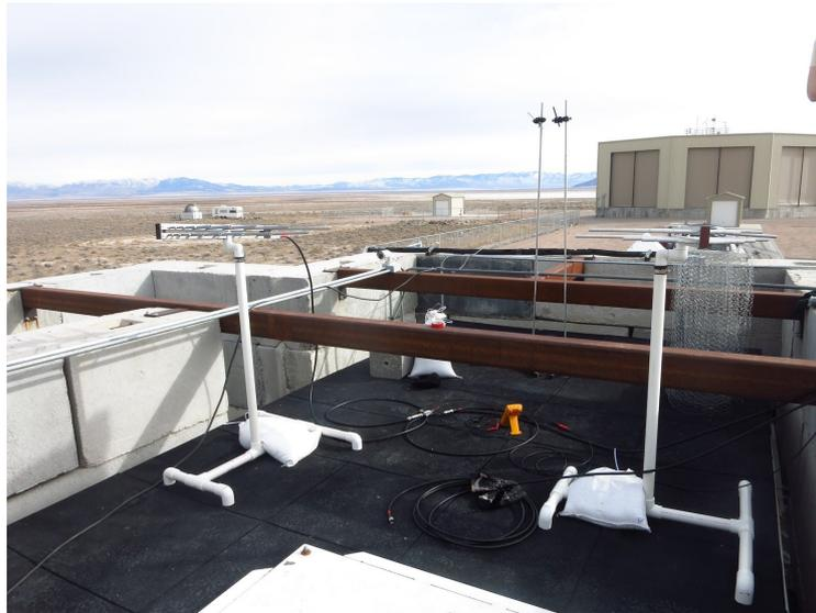
**Figure 2:** A front view of the LPDA set-up, consisting out of two EMCO LPDAs. During the experiment, the antennas were shielded by an RF absorbing screen.
