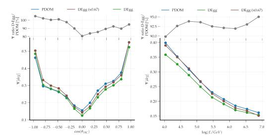
**Figure 4:** The results of the reconstruction SPLINE-RECO, binned in the cosine of the simulated muon direction on the left and binned in the logarithm of the muon energy on the right. Muons with a cosine of -1 are entering the detector from below, those with 1 from above respectively.
