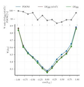
**Figure 3:** The results of the SPEFit reconstruction for both sensors, D-Egg and PDOM binned in the cosine of the simulated muon direction. The D-Egg effective area is scaled down by a factor of 0.67 to match the PDOM effective area. Muons with a cosine of -1 are entering the detector from below, those with 1 from above respectively.
