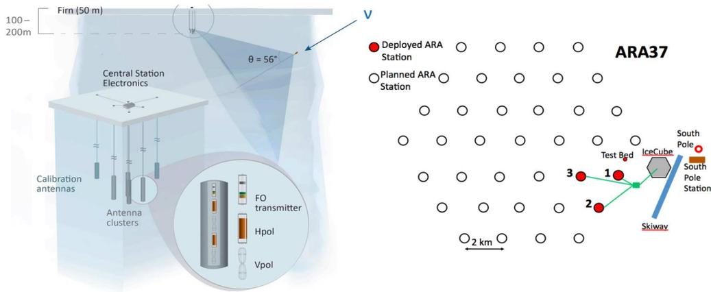
**Figure 1:** Left: ARA station design (see text). Right: ARA plan. Three stations ARA-4,5,6 are scheduled for deployment in 2017/18. Data from ARA-2,3 are discussed in this proceeding.
