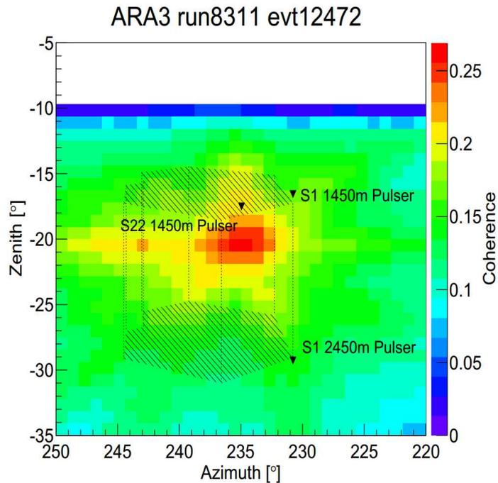
**Figure 5:** Reconstruction of the “sky” position of ICS22 as seen from ARA-3. The methods are described in the ARA analysis presentation to this conference[.]. This reconstruction uses just the Vpol QD rays, but otherwise assumes the station and array geometry and icemodel described herein. The raytracing for reconstruction is table driven, as described in [9].
