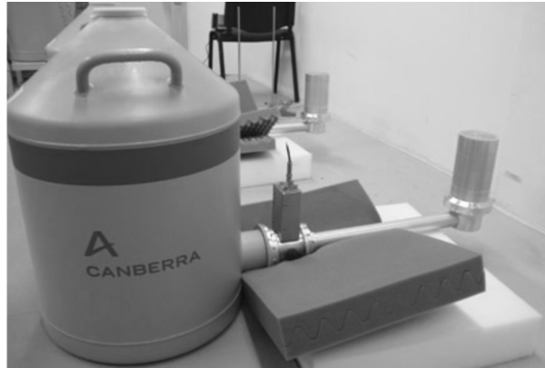
Figure 6: Picture of the Ge detector without shielding in Canfranc.
