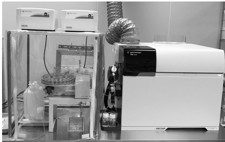
Figure 1: Picture of the ICP-MS “Agilent7900” in Kamioka clean room.
