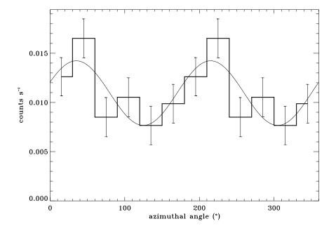
**Figure 3:** Phase-averaged polarisation diagram of the Crab pulsar/nebula obtained by INTEGRAL/IBIS in fall 2015 in the 300-450 keV energy band. The distribution or polarigramme gives the source count rate by azimuthal angle of the Compton scattering. The minimum of the sinusoidal fit indicates a polarisation angle of  $125^{\circ} \pm 15^{\circ}$ , a polarisation fraction of  $89 \pm 28$  and a S/N ratio of 14.
