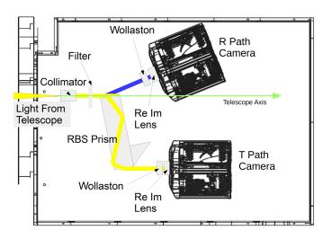
Figure 1: GASP 2D Drawing - showing the layout of the major system components
