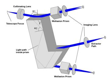
Figure 2: GASP system optical layout.
