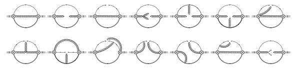
Figure 1: The Feynman diagrams calculated for the correlator (1.1). Single solid lines correspond to light quark propagators whereas double solid lines correspond to heavy quark propagators. All Feynman diagrams are drawn using JaxoDraw [8]
