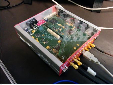
Figure 3: On the left: picture of the SAMPIC chip installed in the development board used for the tests. On the right: RMS of the time difference between two signals generated using a function generator and acquired at 6.4 GSa/s using the SAMPIC evaluation board. The time difference has been computed using three different algorithms and the RMS is shown as a function of the amplitude of the signal [2].
