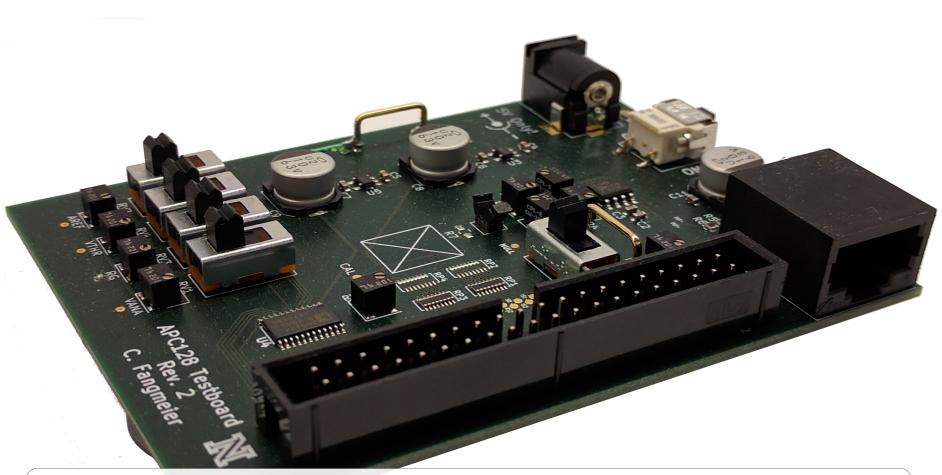
A custom board was developed for gaining familiarity with the APC-128 chip, and for testing different control and readout schemes. It features:
