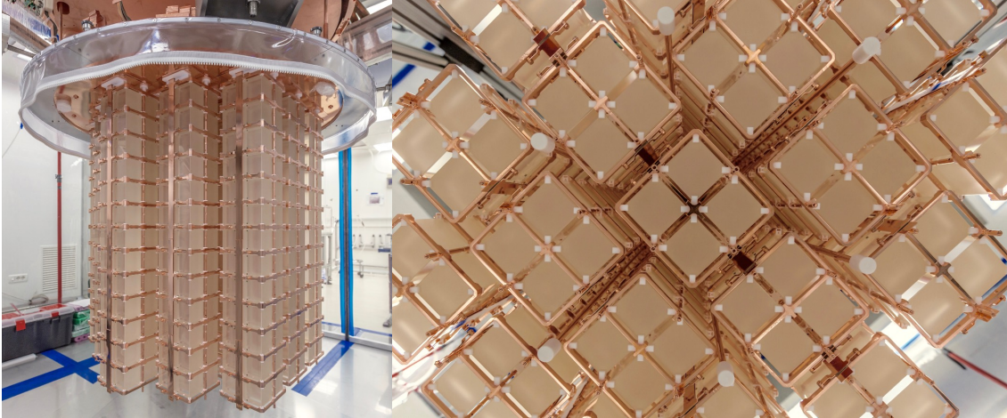
Figure 5: 988 bolometers configured in 19 towers attached on the top supporting plate of the CUORE cryostat (left). Bottom view of the towers, along with six capped guide tubes for the CUORE detector calibration (right).
