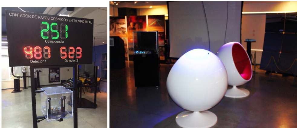
Figure 3: Left: A dual Geiger counter exhibit in the Visitor Center which registers single cosmic-ray muon counts and 2-fold coincidences. Right: Two “pods” in the renovated Visitor Center in which visitors can listen to an informative program about the Observatory.
