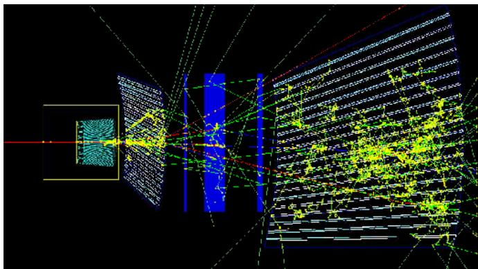
**Figure 4:** GEANT4 simulation of the sPHENIX calorimeter prototypes in the FNAL test beam facility
