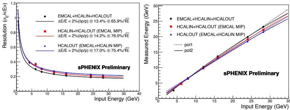
Figure 6: Preliminary energy resolution for the calorimeter setup
