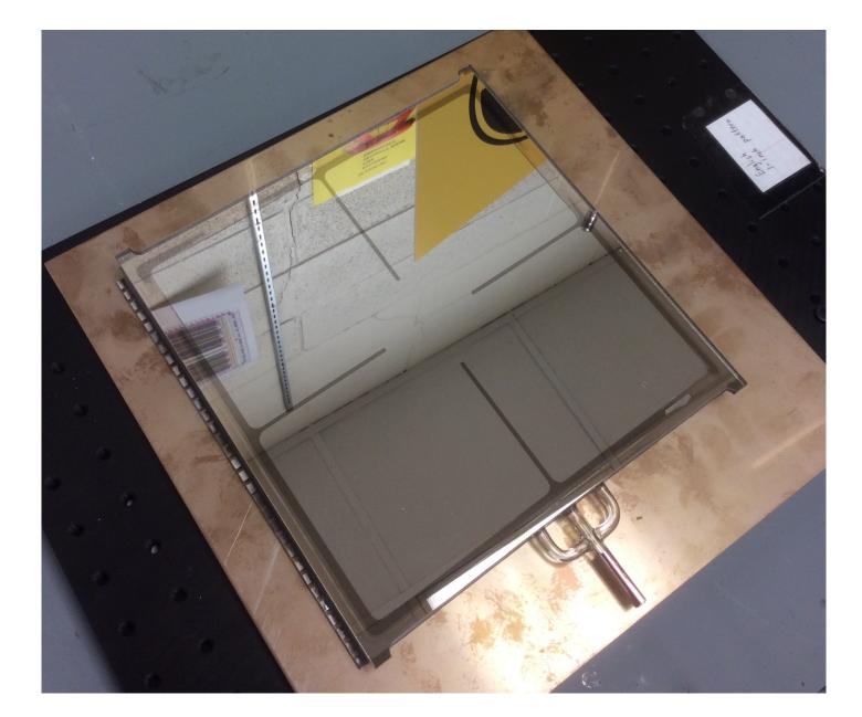
Figure 1: Top-down view of a sealed, LAPPD photo-detector "tile" made by the team at University of Chicago
