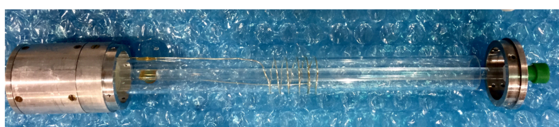
Basis for new plunging probe design: an absolute calibration probe used in the previous experiment, BNL E821 (aluminum housing removed)
