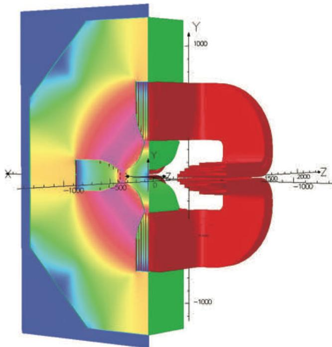
**Figure 5:** Simulated magnetic-field map of the Q1 magnet of the  $S - 2S$  spectrometer system.
