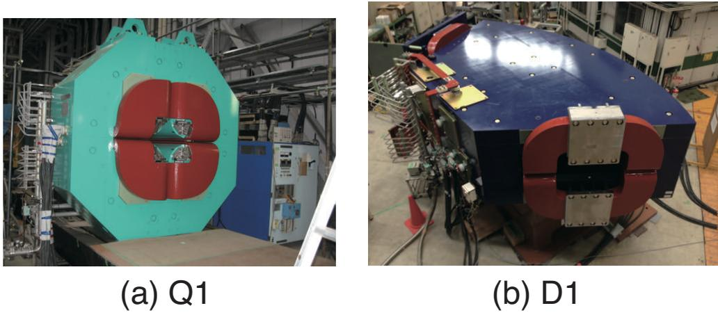
**Figure 4:** Pictures of the (a) Q1 and (b) D1 magnets of the  $S - 2S$  spectrometer system.
