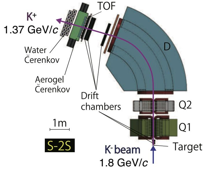
**Figure 3:** Schematic view of the S-2S spectrometer system.
