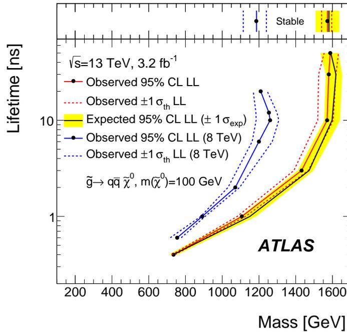
**Figure 3:** Excluded range of lifetimes as a function of gluino  $R$ -hadron mass. The expected lower limit (LL), with its experimental  $\pm 1\sigma$  band, is given with respect to the nominal theoretical cross-section [2]. The observed 95% LL obtained at  $\sqrt{s} = 8$  TeV [3] is also shown for comparison.
