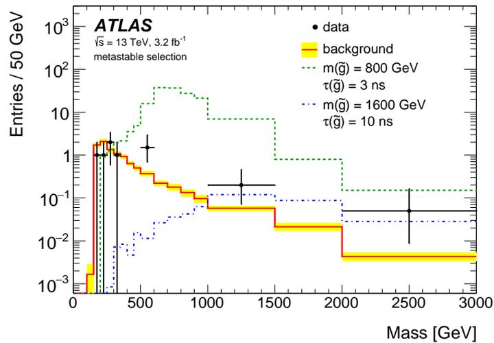
**Figure 2:** Mass distribution for data and background for metastable particle searches. The yellow band around the background estimation includes both the statistical and systematic uncertainties. Also shown are two examples for signals as expected for gluino  $R$ -hadrons in the explored mass range [2].
