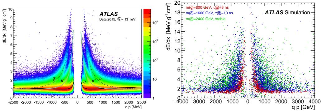
**Figure 1:** (left) Distribution of  $dE/dx$  versus signed momentum for minimum bias 2015 collisions, with tracks reconstructed down to  $p_T$  of 100 MeV. The distributions of the most probable value for the fitted probability density functions of pions (solid), kaons (dashed) and protons (dotted) are superimposed [2]. (right) Simulated distributions of  $dE/dx$  versus signed momentum for  $R$ -hadrons of various masses.
