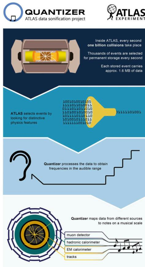
Fig.2: Visual description of the ATLAS Quantizer project.
