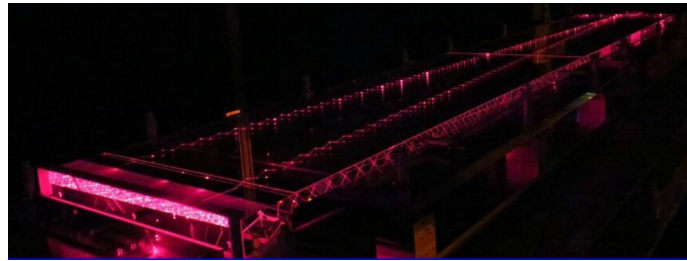
Figure 8: Total internal reflection of laser light inside the last TOP module
