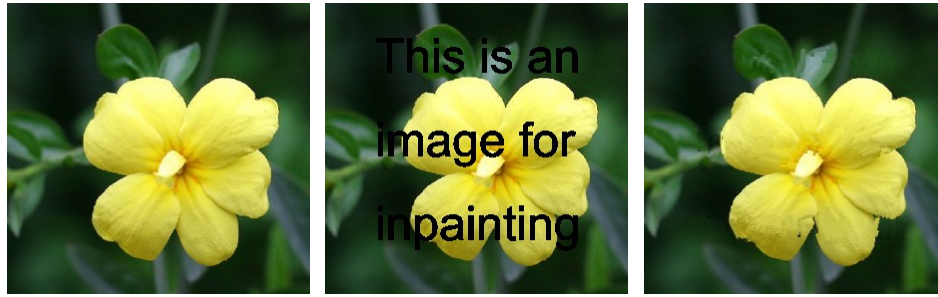
(a)The original image (b) Damaged image (c)The restored image PSNR=33.25 Repair elapsed time 455.92 seconds
