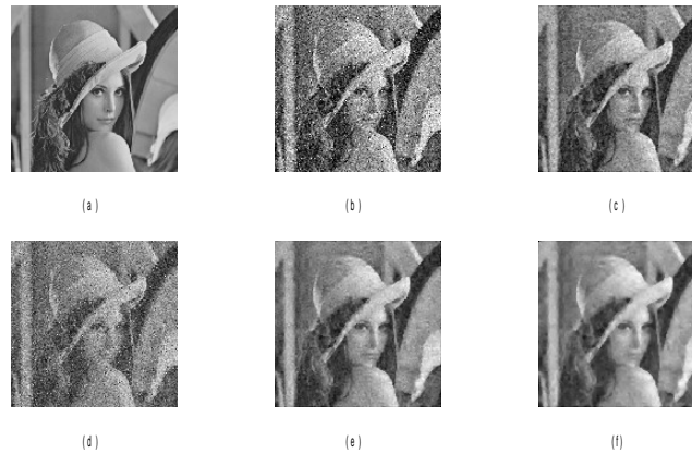
Figure 2 : Results of Different De-noising Algorithms of Lena: (a) Original Image; (b) Noisy Image; (c)Median Filter; (d) Wavelet Transform De-noising; (e) Wavelet Transform and 3*3 Median Filter ; (f)Wavelet Transform and 5*5 Median Filter( \sigma = 0.02 , \rho = 0.02 )
