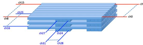
**Figure 9:** Configuration of scintillator bars and corresponding CITIROC channel numbers.
