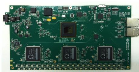
**Figure 7:** First prototype of the Baby MIND Front End Board.
