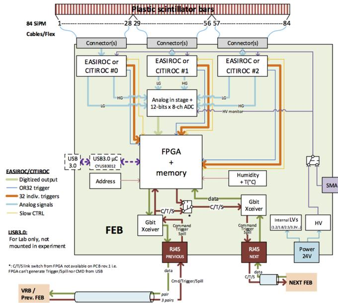
**Figure 6:** Baby MIND readout scheme with an 84-channel implementation per Front-End Board. Up to 96 channels can be connected to one FEB.
