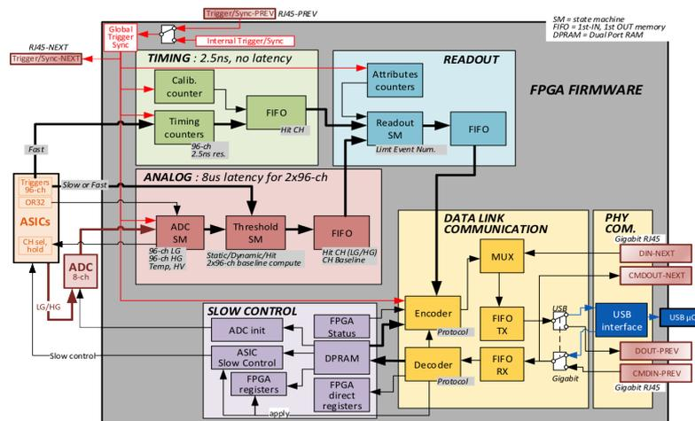
Figure 8: Sketch showing the main blocks of the FPGA firmware.
