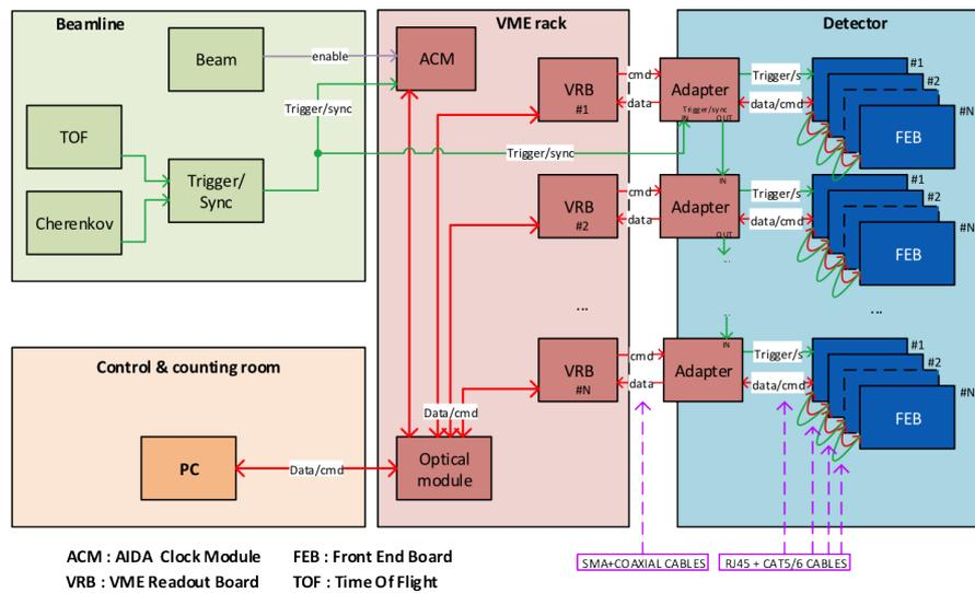
**Figure 3:** Overview of the electronics chain for the Baby MIND detector.
