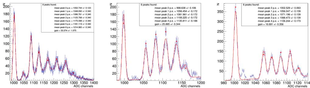
**Figure 10:** Photo-electron peak resolution for a S12571-025C MPPC coupled to a CITIROC chip. Digitized outputs from the high gain path are shown with different feedback capacitance values of 275 fF, 350 fF and 550 fF (settings of 1, 4 and 12 in the CITIROC slow control register and assuming a parasitic capacitance of 250 fF), yielding  $33.37 \pm 1.08$  ADC/p.e.,  $25.89 \pm 0.34$  ADC/p.e. and  $16.69 \pm 0.36$  ADC/p.e. respectively.
