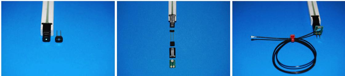
**Figure 1:** Photosensor connectivity. The figure on the left shows the polished fiber end, with a photosensor placed next to it for scale. The figure in the center shows the components that slot into each other to produce the figure on the right.
