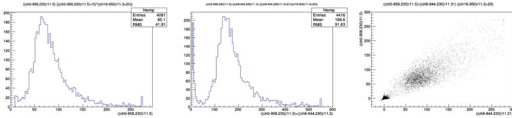
**Figure 12:** Cosmic ray data for one bar, read out from both ends, Ch0 and Ch8, with another bar located underneath used as coincidence, Ch16. Left) light yield from one end, middle) sum of l.y. from both ends, right) 2D plot of l.y. with one channel plotted against the other. All values are photo-electrons.
