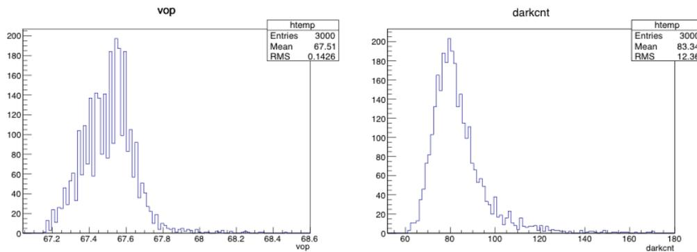
**Figure 2:** Measured properties of the 3000 Type S12571-025C photosensors delivered by Hamamatsu Q1 2015: left) operating voltage in [V], right) dark counts in [kHz].
